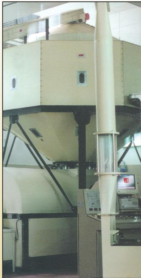
Spietatrice - Silo per caffè tostato - Miscelatore Destoner - Silos for roasted coffee - Mixing machine
